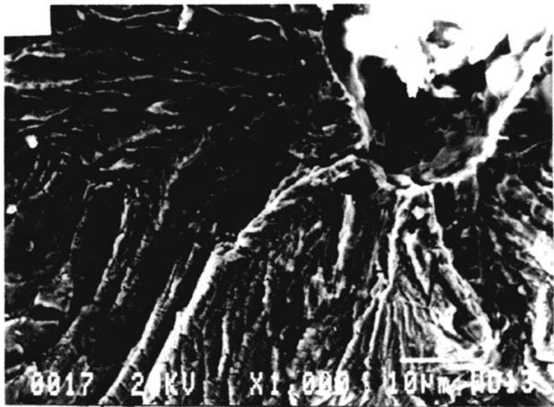
Figure 3 Crack initiation from a pit for a Fe-17Mn-13Cr alloy during CF in a 110°C \text{Cl}^- solution at a plastic strain amplitude \Delta\epsilon_p/2 = 4 \times 10^{-5} and a strain rate \dot{\epsilon} = 10^{-5} \text{ s}^{-1} .
